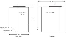
OC Refrigerant Connections: Discharge Line- 3/4", Liquid Line- 1/2"
