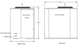
OC Refrigerant Connections: Discharge Line- 5/8", Liquid Line- 1/2"
