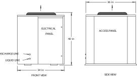
OC Refrigerant Connections: Discharge Line- 1/2", Liquid Line- 3/8"
