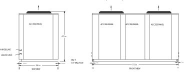
OC Refrigerant Connections: Discharge Line- 3/4" (2), Liquid Line- 1/2" (2)
