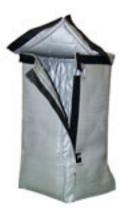
**High-Temp** covers are available if severe conditions or excessive heat is an issue. The material in these covers consists of a quilted fiberglass fabric over a 1" thick fiberglass filler. This material is usable up to 550 degrees F.
